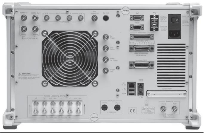
Figure 1-2. VectorStar MS4647 VNA Rear Panel - Equipped with Option 051
